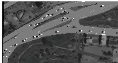
Figure 1: Left: Panchromatic WorldView-2 image of a city with traffic activity. Centre: After the roads have been extracted, PCA produces an output image in which neighbouring dark and bright polygons are visible, an indication of moving vehicles. Right: WorldView-3 image of a rural area showing the detection of a moving vehicle on a dirt road using the same methodology.
