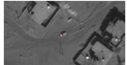
Figure 1: Left: Panchromatic WorldView-2 image of a city with traffic activity. Centre: After the roads have been extracted, PCA produces an output image in which neighbouring dark and bright polygons are visible, an indication of moving vehicles. Right: WorldView-3 image of a rural area showing the detection of a moving vehicle on a dirt road using the same methodology.
