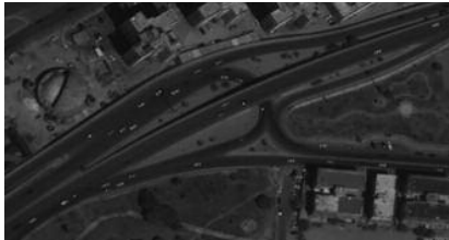
Figure 1: Left: Panchromatic WorldView-2 image of a city with traffic activity. Centre: After the roads have been extracted, PCA produces an output image in which neighbouring dark and bright polygons are visible, an indication of moving vehicles. Right: WorldView-3 image of a rural area showing the detection of a moving vehicle on a dirt road using the same methodology.
